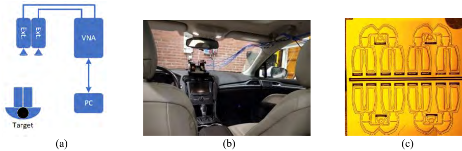
Figure 1. (a) H-band radar system structure, (b) measurement setup in the car cabin, and (c) microscope picture of the fabricated antenna array with micromachined-waveguide distribution network
